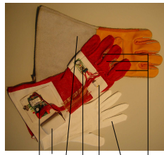
battery Scipio pcb with PromiESD outer glove Tilt sensor rfid scanner inner glove buttons
