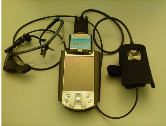
Fig. 2. PDA-Wearable for aircraft maintenance
