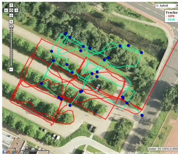
**Fig. 2.** Google Earth view of the parcours with an overlay of the GPS localization data (red), the PDR track (green) and the RFID tags (blue)
